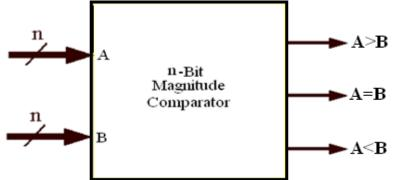
Figure 1. Block Diagram of n-Bit Magnitude Comparator
