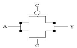
Figure 6. Symbol of Transmission Gate
