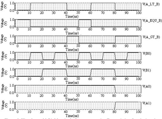
Figure 8. Waveform of 2-Bit Magnitude Comparator using Transmission Gate logic style
