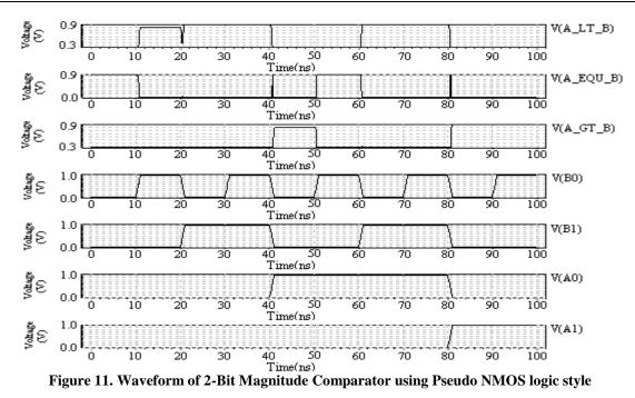
Consider input bits 0100 then according to truth table in output side '1' should be obtained in A>B & rest two output should be '0'. After simulation output waveform (in Fig.11) shows same result as in truth table for these input bit. When input bits are 0101 then expected output in A=B should be '1', & waveform also shows same output as in truth table. Similarly, When input bits are 0110 then expected output in A<B should be '1', & waveform also shows same output as in truth table.
