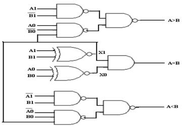
Figure 2. Logic Diagram of 2-Bit Magnitude Comparator
