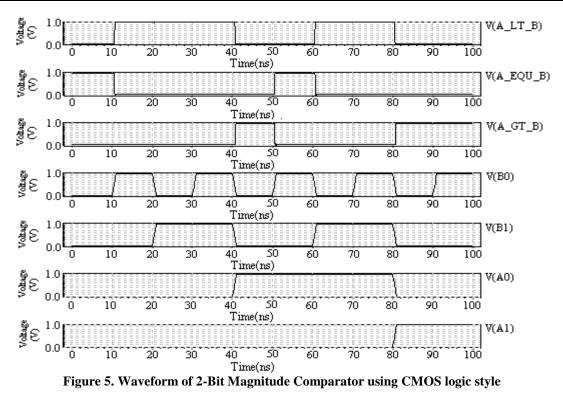
Consider input bits 0100 then according to truth table in output side, '1' should be obtained in A>B & rest two output should be '0'. After simulation output waveform (in Fig.5) shows same result as in truth table for these input bits. When input bits are 0101 then expected output in A=B should be '1', & waveform also shows same output as in truth table. Similarly, When input bits are 0110 then expected output in A<B should be '1', & waveform also shows same output as in truth table.
